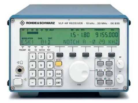
VLF-HF Receiver R&S EK895 with control panel
